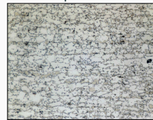
Original microsection of a dual-phase steel
