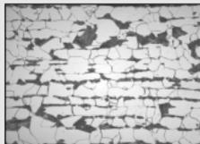
Micro section of a dual-phase steel.
