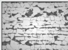
Micro section of a dual-phase steel.
