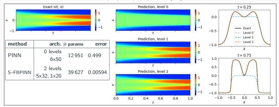
PINN gets stuck at fixed point of the of dynamical system; cf. Rohrhofer et al. (arXiv 2023).
