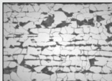
Micro section of a dual-phase steel.
